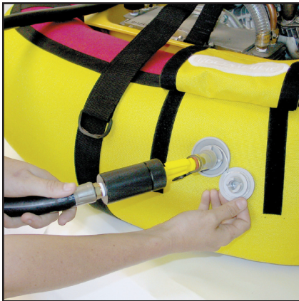
4. Located at the end of the black heat hose is a male QRS fitting which fits snugly into the clear tube. With the compressor running, insert the male QRS fitting into the clear tube and begin filling.
